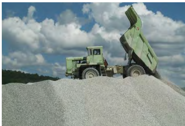
Figure 4.30 Typical Cause of Degradation
