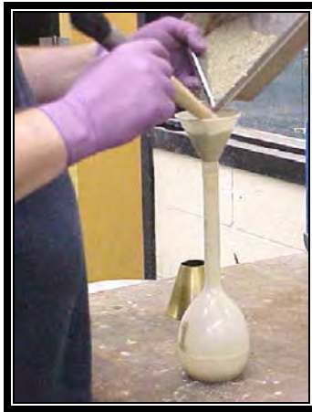
Figure 5 Pouring sand into pycnometer once SSD is achieved
