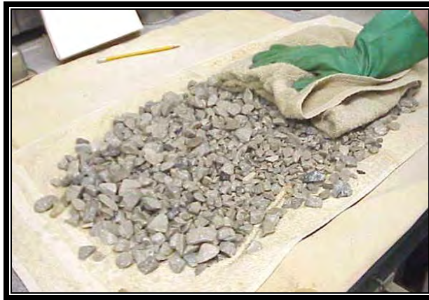
Figure 8 Removing Excess Water
