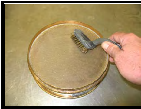
Figure 3 Use Wire brush on Coarse Sieve
