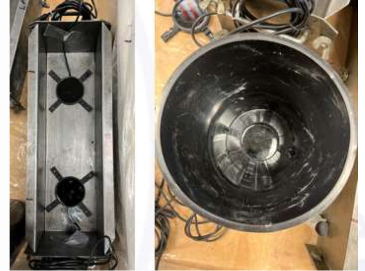
Sensor installed in Lab Trials (slabs, beam, and cylinder)
